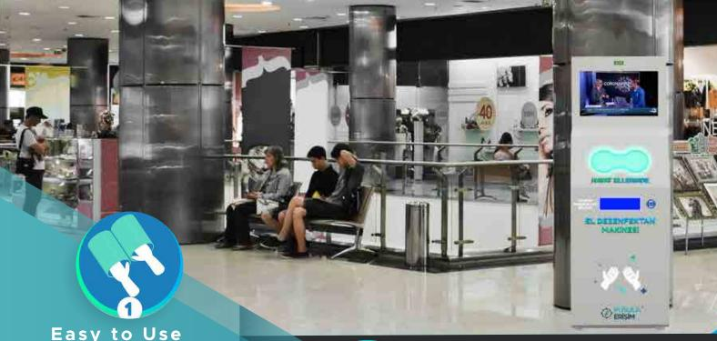
Insert hands in to the sanitizing compartment. Motion sensors will activate the automatic spray, cleaning the hands with anti-bacterial disinfectant mist.
